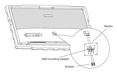
2. Install the unit onto the wall with the mount stud (not included), and then mount it onto the wall.
