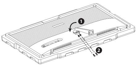
3. Install the base to the stem with 2 screws.
